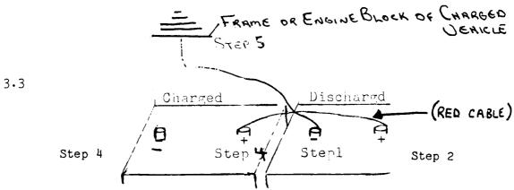
The following steps must be taken when boosting a discharged Battery from a fully charged Battery or an explosion may occur:
